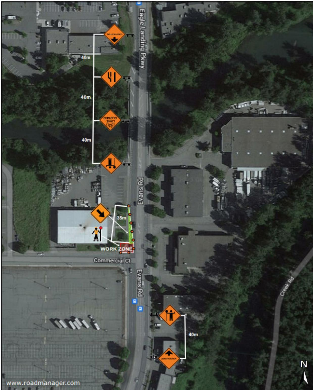
Figure 11.6: Right Lane Closure (Near Side) – Multilane Intersection – Short and Long Duration
